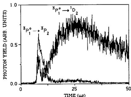
FIG. 4. Time sequential behavior of the  $^3P_1^o \rightarrow ^3P_2$  transition at 405.8 nm and  $^3P_1^o \rightarrow ^1D_2$  at 722.9 nm recorded simultaneously 10 mm downstream from the nozzle exit by two PMTs following initiation of 3 mg of  $Pb(N_3)_2$  at  $t = 0$ . The photon yields are corrected for the wavelength response of the detection system.
