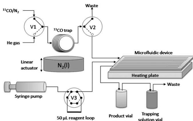
Figure 2. Schematic of the microfluidic  $^{11}\text{C}$  carbonylation setup.
