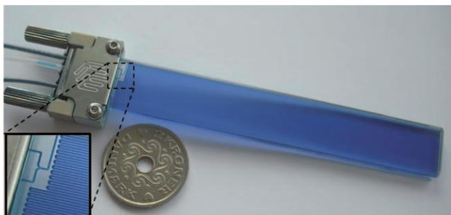
Figure 1. Microfluidic device used for  $^{11}\text{C}$  carbonylation reactions. The device is filled with a blue dye to emphasise the channel structure. Bottom left hand quadrant shows a close-up of the inlet channels. See the Supporting Information for details of the microfluidic reactor design and substrate solution preparation.
