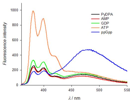
**Figure 2.** Fluorescence emission spectra of PyDPA (20  $\mu$ M in 1 mM HEPES pH 7.5) alone and upon addition of each nucleotide and ppGpp (7  $\mu$ M). Ex = 344 nm.
