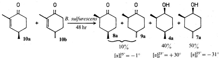
FIG. 4. Microbiological Reduction of (+)-2,4-Dimethylcyclohex-2-en-1-ones by *Beauveria sulfurescens*.
