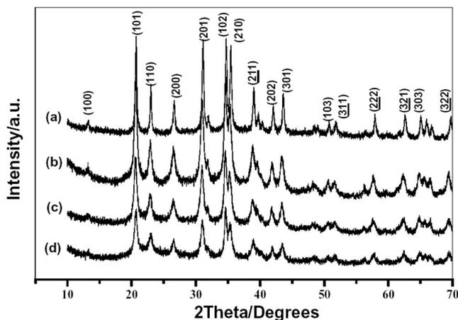
Fig. 1. XRD patterns of the products prepared by reacting  $\text{Mg}_2\text{Si}$  with  $\text{NH}_4\text{Cl}$  for 10 h in an autoclave at (a) 450°, (b) 500°, (c) 550°, and (d) 600°C.
