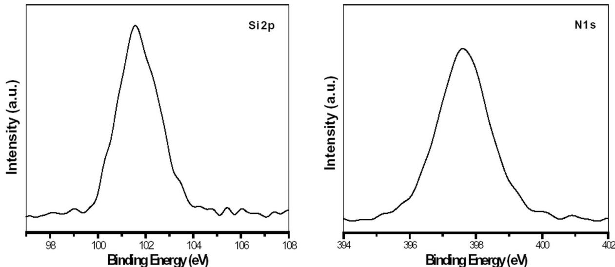
Fig. 3. XPS spectra of the as-prepared  $\alpha$ - $\text{Si}_3\text{N}_4$  powders.
