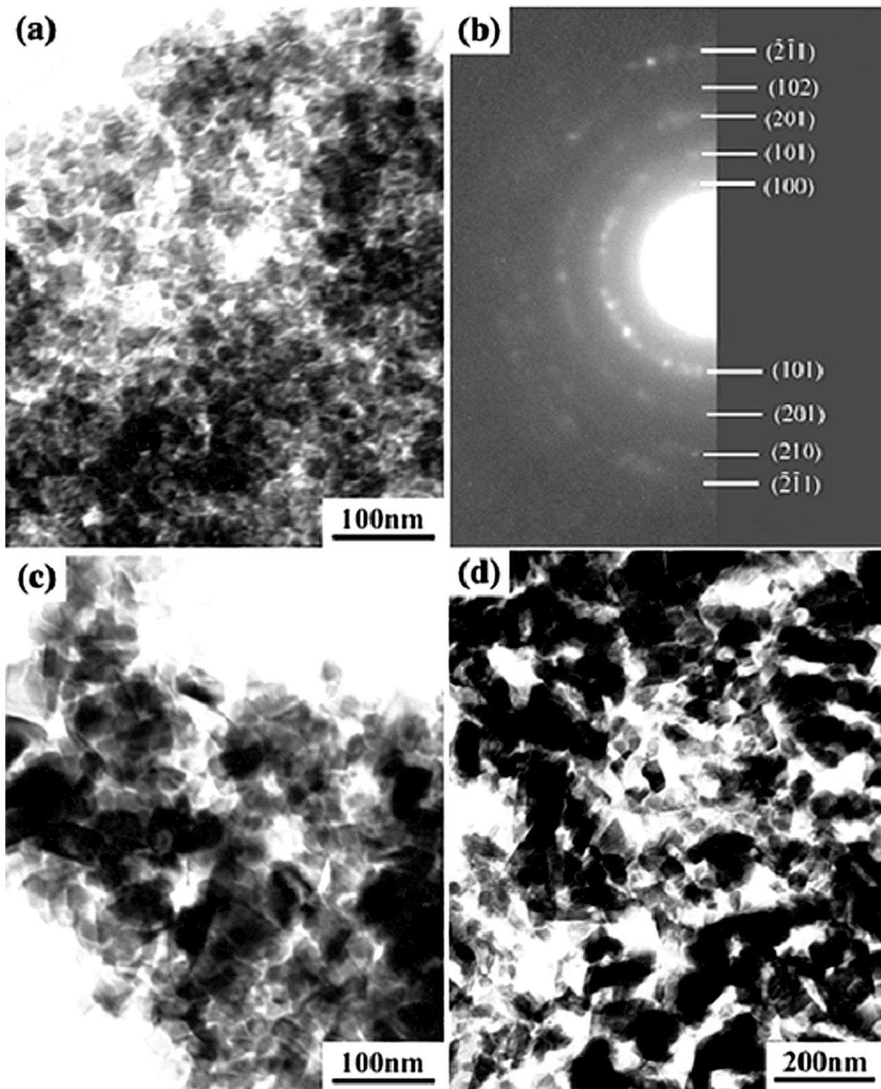
**Fig. 2.** TEM images and selected area electron diffraction (SAED) patterns of the  $\alpha$ - $\text{Si}_3\text{N}_4$  samples prepared at (a and b)  $450^\circ$ , (c)  $500^\circ$  and (d)  $550^\circ\text{C}$ .
