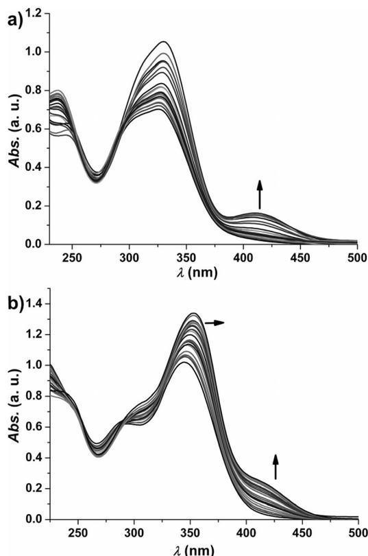
Figure 3. Changes in the UV/Vis spectra of 3.3  $\mu\text{M}$  solutions of **S1** (a) and **S2** (b) upon addition of increasing amounts of cyanide (0.1 to 20 equiv.) in THF/water.
