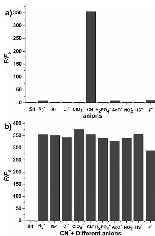
Figure 7. Fluorescence responses of (a) **S1** (3.3  $\mu\text{M}$ ) upon addition of various anions (5 equiv.) in THF/water solution, (b) **S1** (3.3  $\mu\text{M}$ ) to  $\text{CN}^-$  (1 equiv.) containing various anions (5 equiv.).  $\lambda_{\text{ex}} = 326 \text{ nm}$ , Slit: 2.5 nm/2.5 nm.
