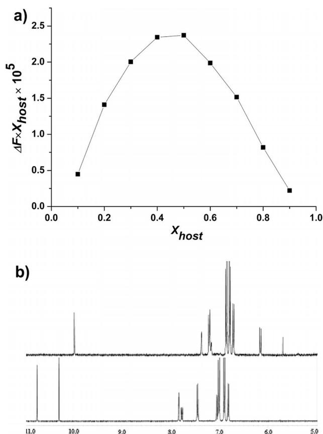
Figure 8. (a) Job plot of **S1** with  $\text{CN}^-$ ; (b)  $^1\text{H}$  NMR spectral change of the dosimeter upon addition of cyanide anions: (below) sensor **S1** only, and (above) sensor and  $\text{CN}^-$  (10 equiv.) in  $[\text{D}_6]\text{DMSO}$ .
