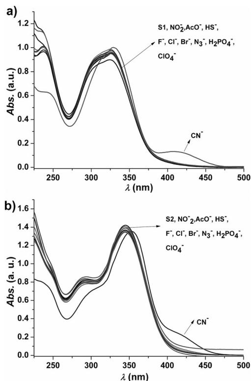
Figure 1. UV/Vis spectra of 0.1 mM solutions of (a) **S1** and (b) **S2** in THF/water mixture (95:5) upon addition of different anions (5 equiv.).
