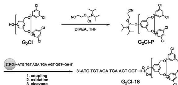
Scheme 1 The solid phase synthesis of the  $G_2Cl$ -18 hybrid.
