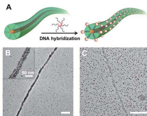
**Fig. 2** (A) Schematic illustration of the hybridization of DNA modified AuNPs with  $G_2Cl-18$  nanofibers. TEM images of the hybridization of  $G_2Cl-18$  nanofibers with 5 nm AuNPs containing (B) complementary ssDNA and (C) non-complementary ssDNA. Inset is the enlarged image. The scale bar is 200 nm.
