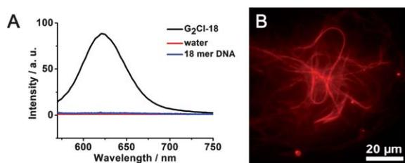
**Fig. 3** (A) The fluorescent emission spectra of Nile Red in aqueous solution in the presence or absence of G<sub>2</sub>Cl-18 hybrid and (B) the fluorescent image of the nanofibers after Nile Red encapsulation.
