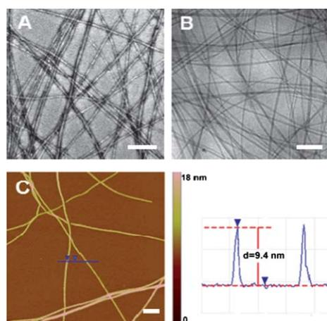
**Fig. 1** Images of nanofibers formed by self-assembly of  $G_2Cl-18$  in aqueous solution. (A) Negatively stained TEM image, (B) cryo-TEM image and (C) AFM image, including cross-section height analysis. The scale bar is 200 nm.
