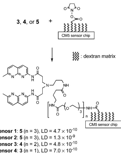
**Scheme 2.** Immobilization of naphthyridine dimers having different ligand density (LD, fmol·nm<sup>-2</sup>) and lengths of a PEO linker on to the dextran coated gold surface.
