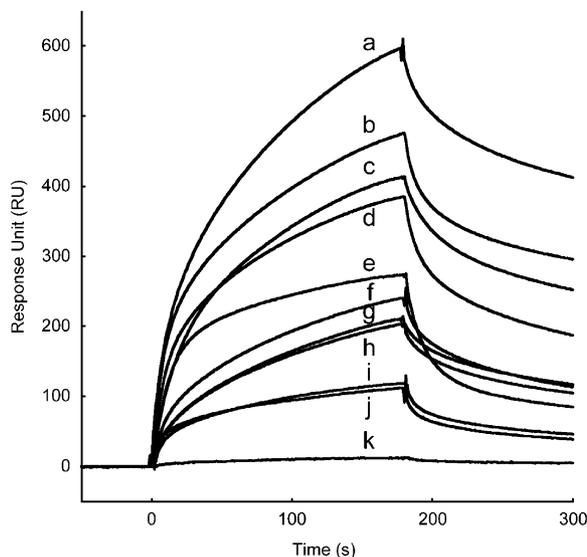
**Figure 4.** Sensorgrams obtained for the binding of XYZ/X'Y'Z' to **Sensor 1** at a concentration of 1 μM duplex. Binding was measured for 180 s and dissociation for 120 s. Key: (a) GGC/CGG, (b) CGG/GGC, (c) CGC/GGG, (d) TGG/AGC, (e) TGA/AGT, (f) AGG/TGC, (g) TGC/AGG, (h) AGC/TGG, (i) AGA/TGT, (j) AGT/TGA, (k) CGG/GAC (GA mismatch).
