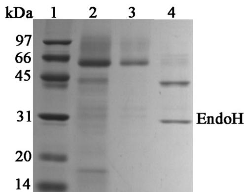
**Fig. 2.** SDS-PAGE analysis of the purified recombinant XYN10C1. Lane 1, standard protein molecular weight markers; lane 2, the culture supernatant; lane 3, the purified recombinant XYN10C1; lane 4, the purified recombinant XYN10C1 after deglycosylation with Endo H.
