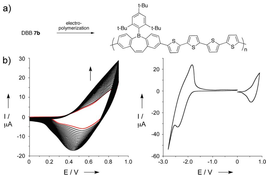
**Figure 8.** Electrochemical polymerization data for poly(**7b**). (a) Growth curve showing multiple CV traces of monomer **7b** and (b) cyclic voltammogram of the resulting polymer. CVs were obtained in 0.1 M *n*-Bu<sub>4</sub>NPF<sub>6</sub>/THF with polymer growth done in a 2.5 mM solution of **7b**. All potentials are reported relative to Ag/Ag<sup>+</sup>.
