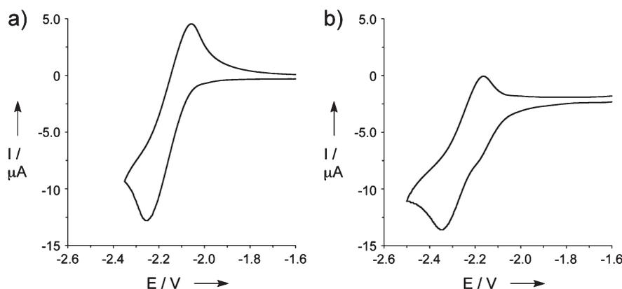
**Figure 7.** Cyclic voltammetry of **7a** (a) and **7e** (b). CVs were acquired in 2.5 mM solutions of analyte in 0.1 M  $n\text{Bu}_4\text{NPF}_6/\text{THF}$  and are reported relative to  $\text{Ag}/\text{Ag}^+$ .
