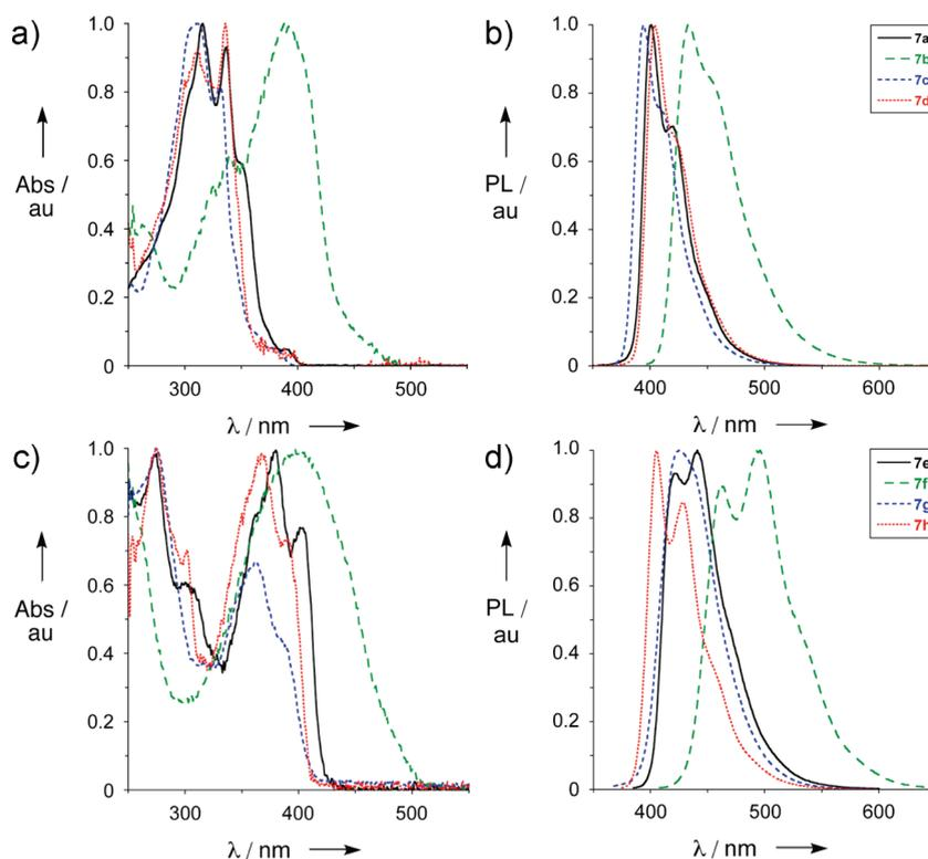
**Figure 4.** Normalized UV-vis data for (a) *para* substituted DBBs 7a–d and (c) *meta* substituted DBBs 7e–h and normalized photoluminescence data for (b) *para* substituted DBBs 7a–d and (d) *meta* substituted DBBs 7e–h. UV-vis and PL spectra were acquired in CHCl<sub>3</sub> at room temperature. The legends for panels a and b are shown in panel b, and those for panels c and d are shown in panel d.
