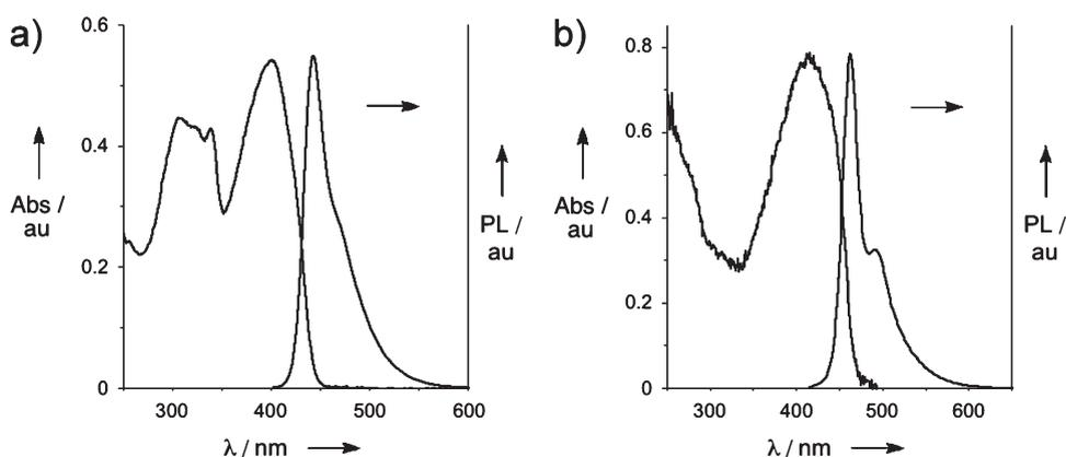
**Figure 6.** UV-vis and photoluminescence data for **8a** (a) and **8b** (b). UV-vis and PL spectra were acquired in  $\text{CHCl}_3$  at room temperature, with excitation at 397 nm (a) and 410 nm (b).
