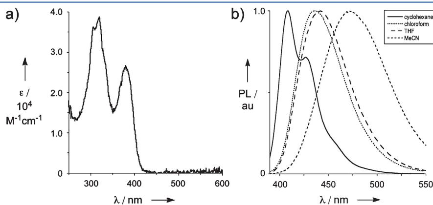
**Figure 5.** UV-vis (a) and photoluminescence (b) data for **7i**. UV-vis was acquired in  $\text{CHCl}_3$ , and PL spectra were acquired in cyclohexane,  $\text{CHCl}_3$ , THF, and MeCN at room temperature, with excitation at 379.
