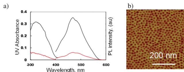
**Figure 1.** a) UV-vis (left) and luminescence (right) spectra of **3d** in a thin film before (black) and after (red) annealing at 180 °C for 24 h. b) AFM image (phase mode) of the thin film of **3d**.
