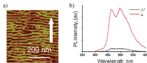
**Figure 2.** a) AFM image (phase mode) of the thin film of **3d** prepared by the friction transfer method. The arrow shows the drawing direction. b) Luminescence spectra of the thin film with perpendicular (upper) and parallel (lower) polarized light (excitation wavelength: 330 nm).
