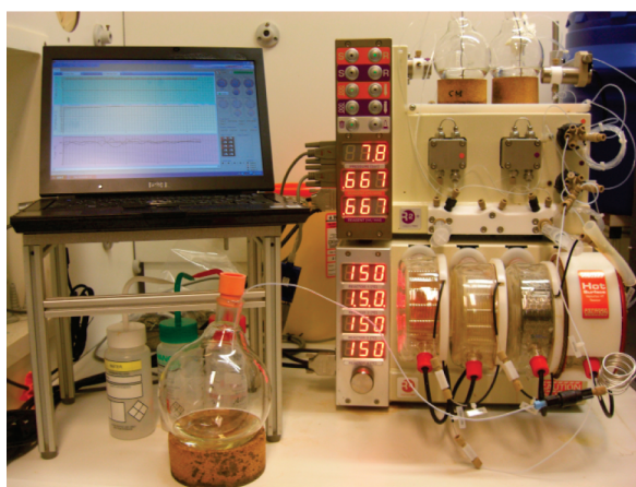
Figure 1. Vapourtec R4 flow reactor setup.
