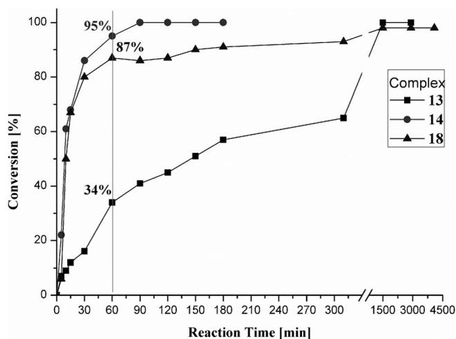
Figure 4. Conversions of 4-bromotoluene in the Suzuki–Miyaura cross-coupling with **13**, **14** and **18**. Reaction conditions: aryl bromide (2 mmol), phenylboronic acid (3 mmol), [Pd] (1 mol-%),  $K_3PO_4$  (3.9 mmol), *n*-dodecane (internal standard), toluene (10 mL), argon. Stated conversions were obtained after 60 min.
