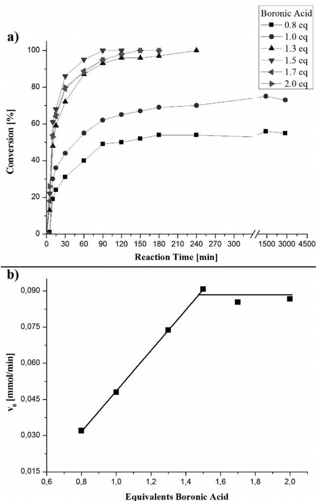
Figure 2. (a) Conversion of 4-bromotoluene in the Suzuki–Miyaura cross-coupling reaction with different amounts of phenylboronic acid. (b) Initial reaction rates ( $v_0$ ) of Suzuki–Miyaura cross-coupling reactions of 4-bromotoluene with different equivalents of phenylboronic acid. Reaction conditions: aryl bromide (2 mmol), phenylboronic acid, **14** (1 mol-%),  $K_3PO_4$  (3.9 mmol), *n*-dodecane (internal standard), toluene (10 mL), argon.
