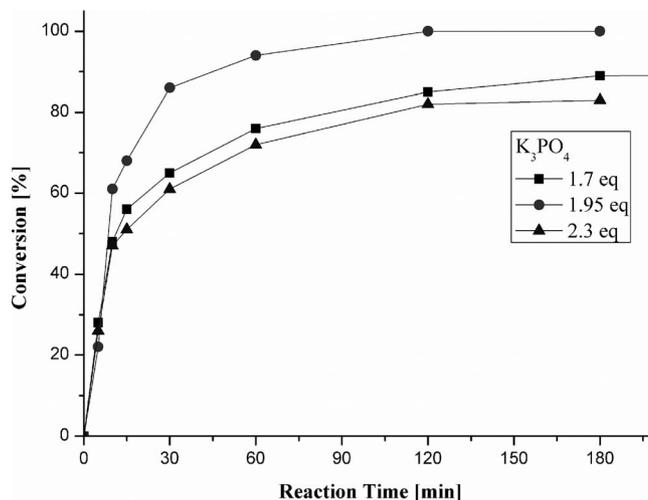
Figure 3. Conversions of 4-bromotoluene in the Suzuki–Miyaura cross-coupling with different amount of  $K_3PO_4$ . Reaction conditions: aryl bromide (2 mmol), phenylboronic acid (3 mmol), **14** (1 mol-%),  $K_3PO_4$ , *n*-dodecane (internal standard), toluene (10 mL), argon.
