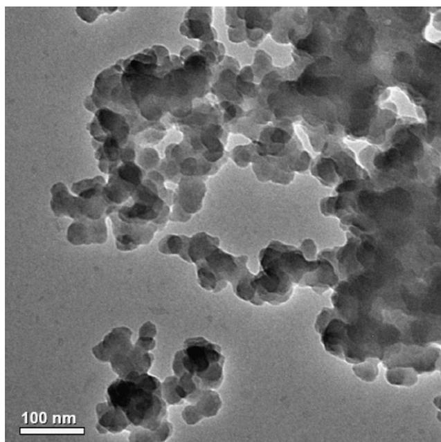
**Figure 5.** TEM image unstained of Gd(CA-NE3TA) ( $10 \mu\text{M}$  aqueous solution).
