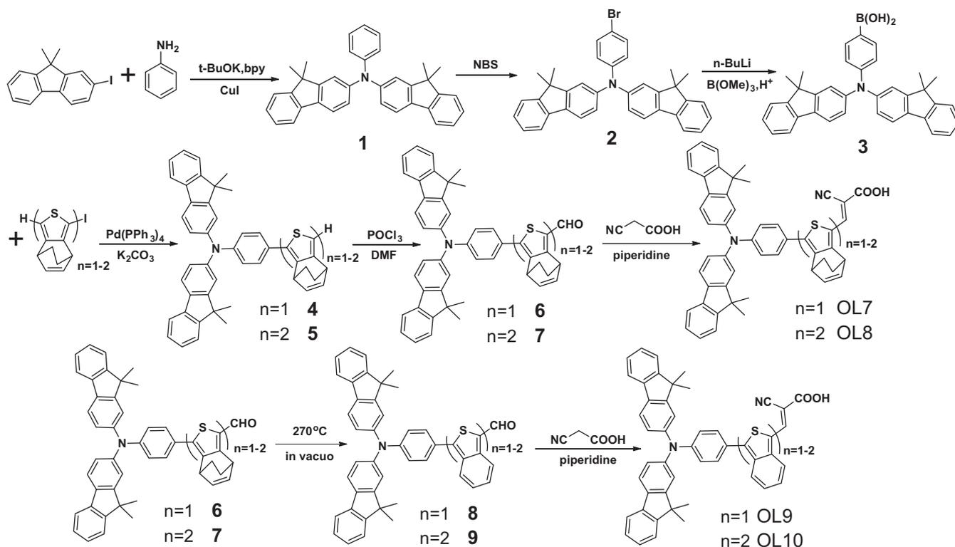
Scheme 1. Synthetic procedure for dyes **OL7–OL10**.
