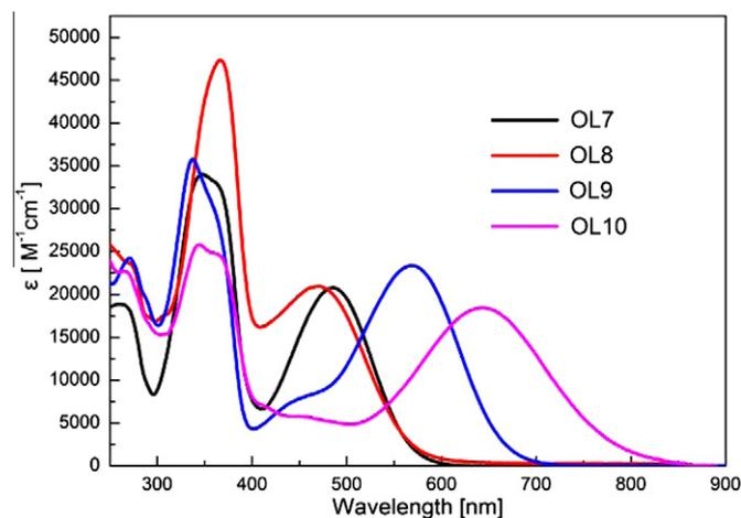
Figure 1. UV-vis absorption spectra of dyes **OL7–OL10** measured in  $\text{CH}_2\text{Cl}_2$ .
