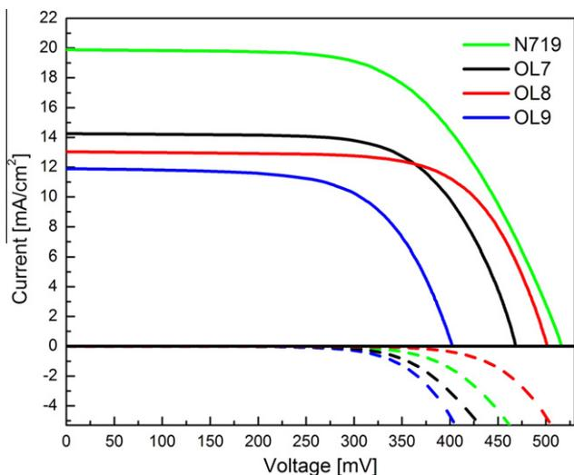
**Figure 4.**  $J$ - $V$  curves of DSSCs based on **OL7-OL9** and **N719** under irradiation of  $100 \text{ mW/cm}^2$  at 1.5AM sunlight condition.
