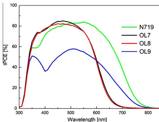
**Figure 3.** The incident photon-to-current conversion efficiency spectra for DSSCs based on **OL7–OL9** and **N719**.
