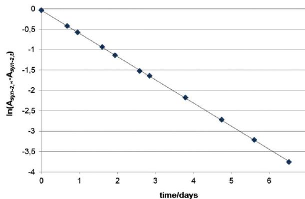
Fig. 7 First-order kinetic plot for the conversion of *anti*-**2** to *syn*-**2** in  $\text{C}_6\text{D}_6$  at 50 °C monitored by  $^{31}\text{P}$  NMR spectroscopy.
