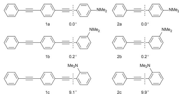
Fig. 6 Calculated dihedral angles between the neighbouring benzene rings in the optimised geometries of **1a–c** and **2a–c**.
