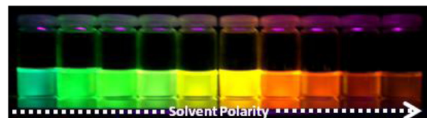
Fig. 3. Top: Normalized absorption and photoluminescence spectra of 2 . Bottom: Illustration of fluorescent polarity probe behavior of compound 2 ( \lambda_{\text{exc}}=365\text{ nm} ).
