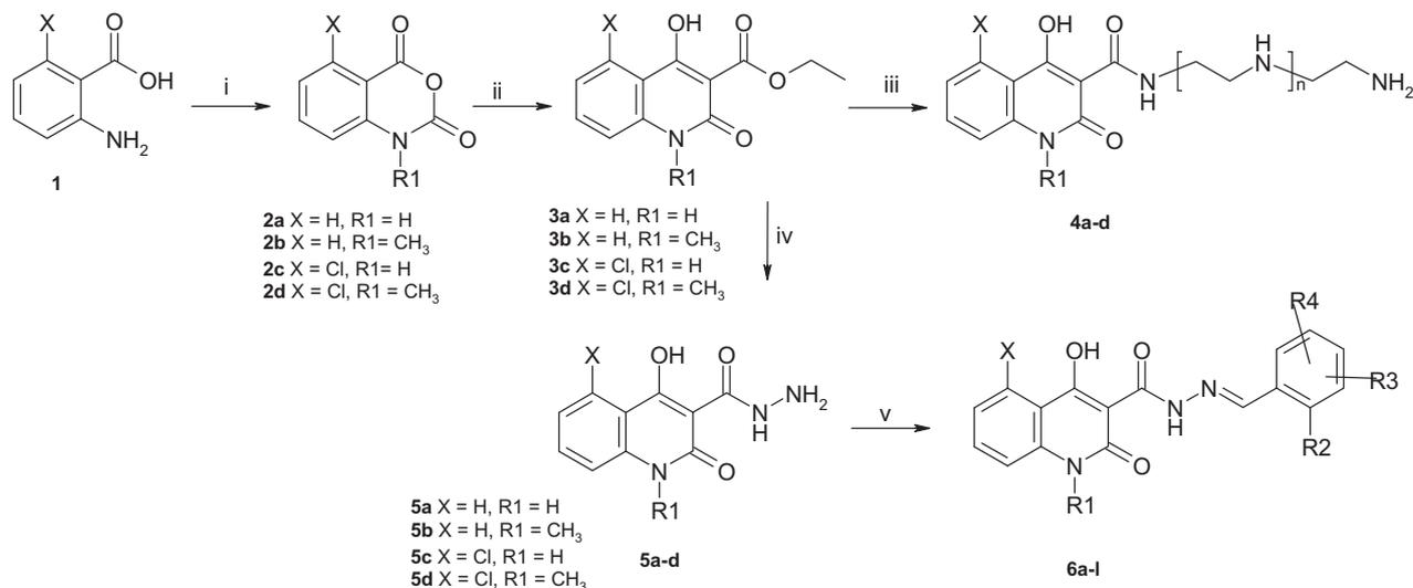
Scheme 1. Synthesis of designed inhibitors **4a–d** and **6a–l**. Reagents and conditions: (i) triphosgene, dioxane, 3 h, 0 °C; (ii) diethyl malonate, NaH, DMF, 2 h, 30, 100 °C; (iii) triethylenetetramine or diethylenetetramine, xylene, 2 h, 150 °C; (iv) hydrazine, MeOH, 30 min, 100 °C; (v) corresponding benzaldehyde, *o*-phosphoric acid, DMSO, 3 h, 100 °C.
