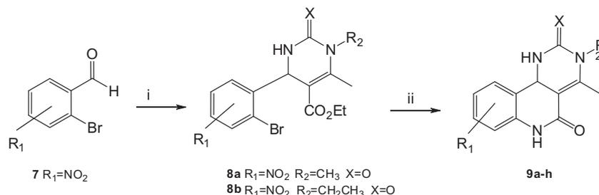
**Scheme 2.** Synthesis of designed inhibitors **9a–h**. (i) H<sub>2</sub>NXNR, H<sub>3</sub>BO<sub>3</sub>, AcOH, ethyl acetoacetate; (ii) NH<sub>3</sub> 28%, 250 °C, 10 bars.
