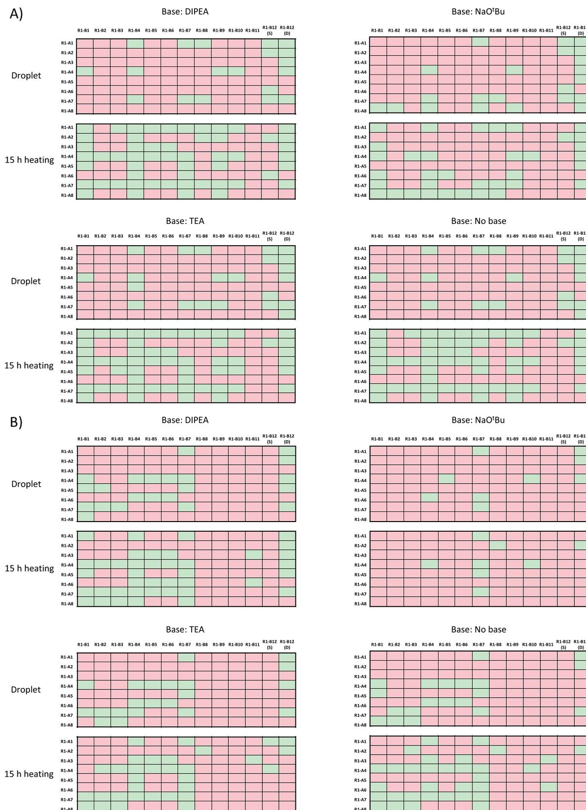
**Figure 1.** Heat map of 1536 reactions from round 1 of the  $S_NAr$  HTE using MeOH with 1% FA as DESI spray solvent under droplet/thin film or bulk microtiter plate conditions at 150 °C for 15 h using four different bases. (A) Reaction solvent, NMP; (B) reaction solvent, 1,4-dioxane. Green cells represent successful reactions (average product intensity  $\geq 150$  counts). Red cells represent unsuccessful reactions (average product intensity  $< 150$  counts).
