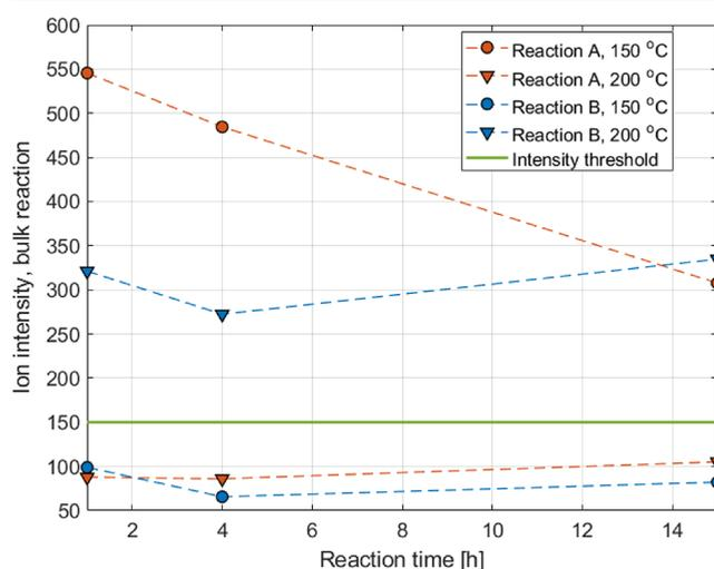
Figure 4. Two representative examples of heated bulk reaction outcomes showing the negative impact of thermal degradation (reaction A) and the positive effects of heating (reaction B). Reaction A: R2-A6, R1-B12(D); base, NaOtBu in NMP. Reaction B: R2-A6, R1-B3; base, DIPEA in NMP. The dashed lines are only to guide the eye.
