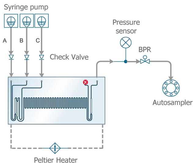
**Figure 5.** Continuous  $S_NAr$  reactions in flow using a Chemtrix glass chip reactor, SOR 3225: A = amine; B = aryl halide; C = DIPEA.
