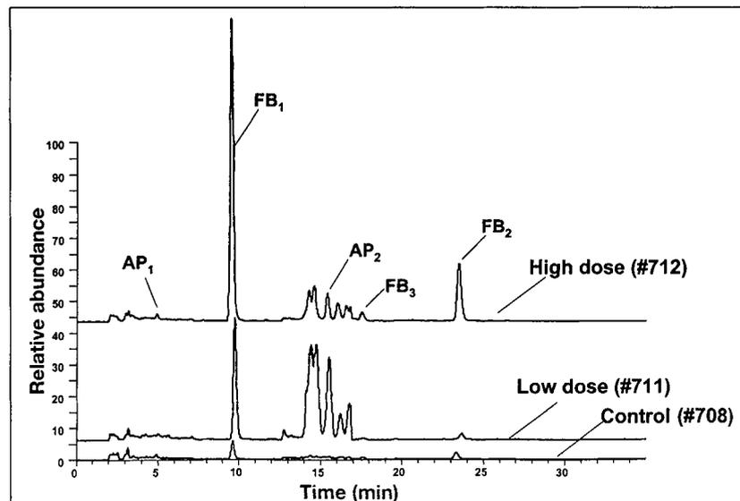
Figure 1. Total ion chromatograms of the hair extracts from nonhuman primates exposed to different levels of toxins showing fumonisin analogues present in hair matrix.
