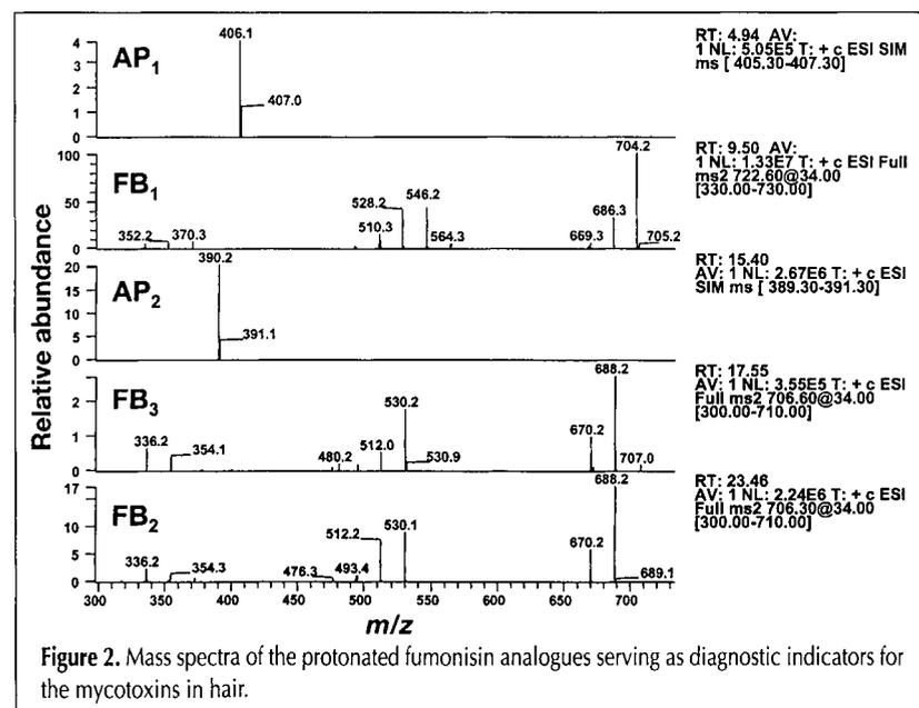
Figure 2. Mass spectra of the protonated fumonisin analogues serving as diagnostic indicators for the mycotoxins in hair.
