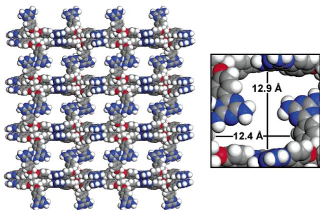
**Figure 3.** Views along the *b* axis of the network constructed from tecton **7**, showing a  $4 \times 4 \times 2$  array of unit cells (left) and an enlarged view of the cross section of a single channel (right). Guests are omitted, and atoms are shown as spheres of van der Waals radii.
