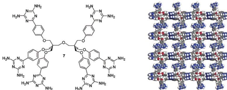
Molecules that associate to form porous networks can be made by attaching multiple hydrogen-bonding sites to suitable cores. Pentaerythritol tetraphenyl ether, a four-armed core, is the progenitor of dendritic derivatives with more arms, including dipentaerythritol hexaphenyl ether **7**. An advantage of such dendritic derivatives is that the resulting networks are held together by larger numbers of intermolecular hydrogen bonds.
