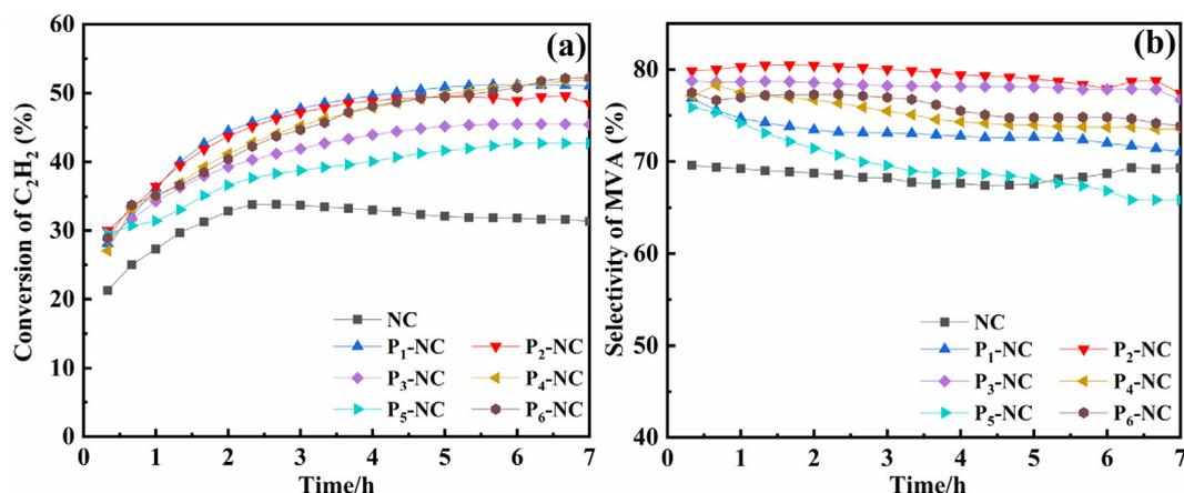
Fig. 2. Catalytic performances of the  $P_x$ -NCs ( $P_1$ – $P_6$ ) on acetylene dimerization: (a) conversion of  $C_2H_2$  and (b) selectivity of MVA. Reaction conditions:  $T = 80\text{ }^\circ\text{C}$ ,  $GHSV(C_2H_2) = 105\text{ h}^{-1}$ ,  $P_x/Cu(I) = 0.05/1.00$ .
