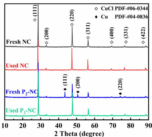
Fig. 3. XRD spectra of the fresh and used NCs and  $P_2$ -NCs after calcination.
