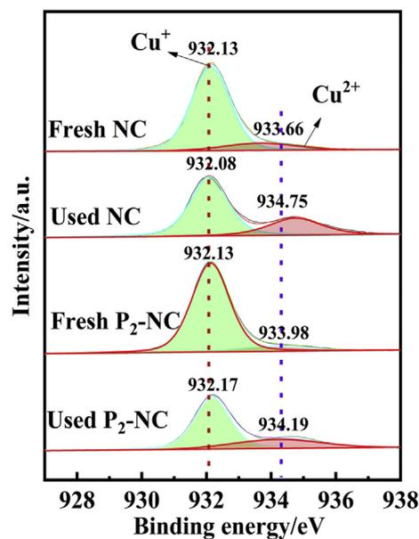
Fig. 5. XPS spectra of Cu 2p<sub>3/2</sub> in the fresh and used catalysts.
