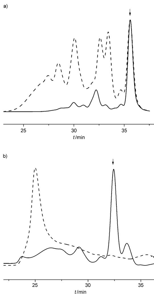
Figure 1. a) The GPC curves of crude product of macrocycle **1** catalyzed by 1.0%  $[\text{Pd}_2(\text{dba})_3]$ +4.0%  $\text{P}(\text{tBu})_3$  (—) and 2.0%  $[\text{Pd}(\text{PPh}_3)_4]$  (-----). b) The GPC curves of crude product of macrocycle **3** catalyzed by 1.0%  $[\text{Pd}_2(\text{dba})_3]$ +4.0%  $\text{P}(\text{tBu})_3$  (—) and 2.0%  $[\text{Pd}(\text{PPh}_3)_4]$  (-----). The sharp peaks marked with arrows represent target macrocycles.
