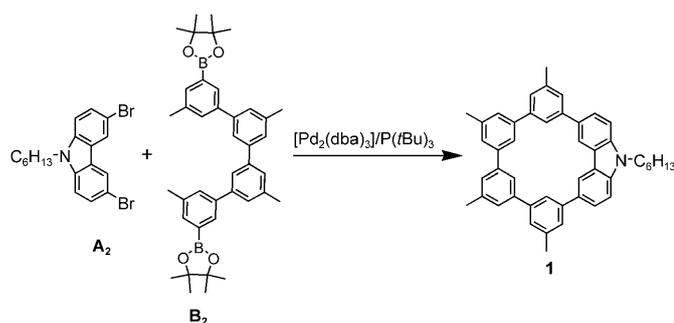
Scheme 1. Synthesis of macrocycle **1** by catalyst-transfer Suzuki–Miyaura coupling reaction.
