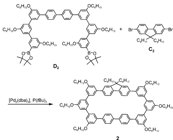
Scheme 2. Synthesis of macrocycle **2** by catalyst-transfer Suzuki–Miyaura coupling reaction.
