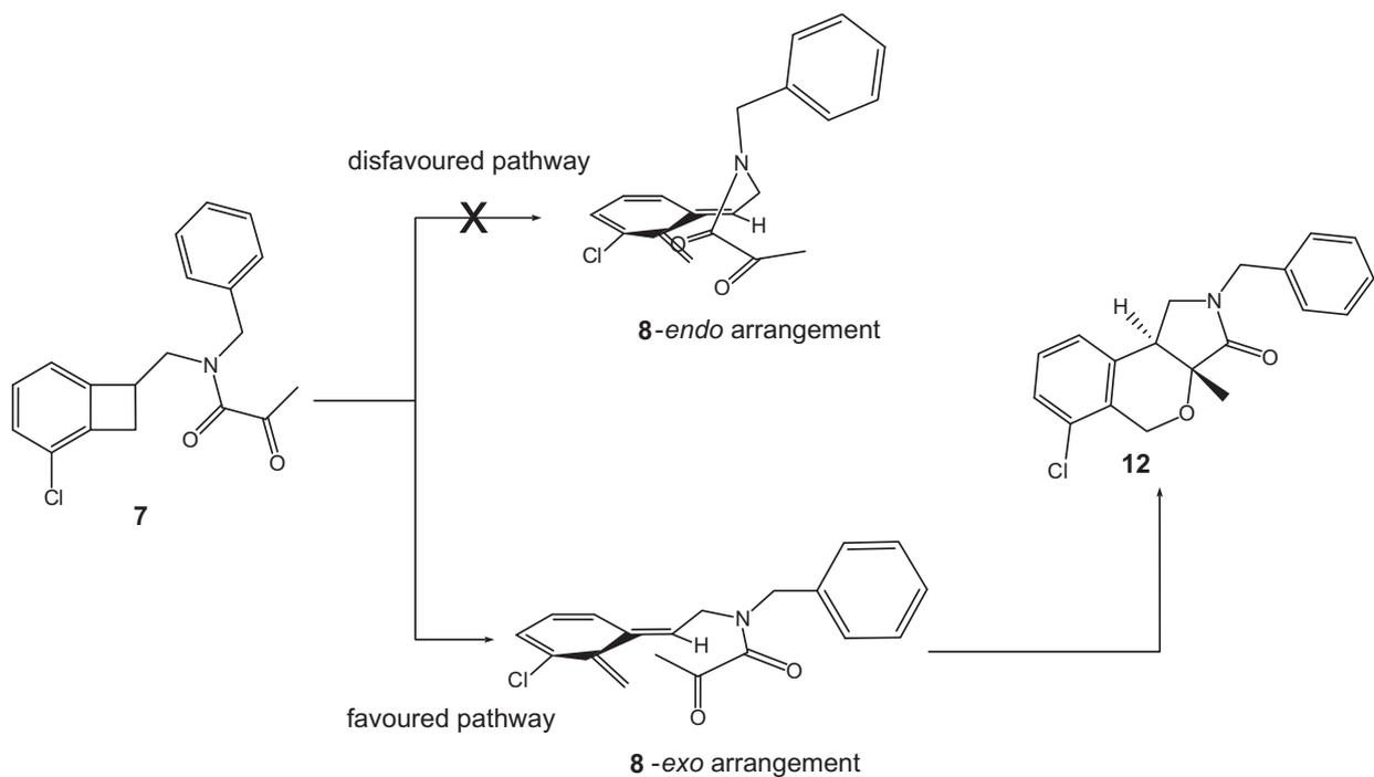
**Figure 3.** Proposed arrangement of the *o*-quinodimethane prior to the Diels–Alder reaction leading to the *trans*-product.
