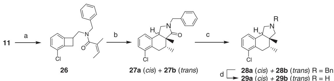
**Scheme 4.** Reagents and conditions: (a) angelic acid, 2,4,6-tripropyl-1,3,5,2,4,6-trioxatriphosphorinane-2,4,6-trioxide,  $\text{Et}_3\text{N}$ , rt, 16 h, 48%; (b) bromobenzene, 190 °C, microwave irradiation, 1 h, 100%; (c) (i)  $\text{BH}_3$ ·THF, THF, reflux, 4 h, (ii) 2 N HCl, **28a** (21%), **28b** (58%); (d) 1-chloroethyl chloroformate, toluene, 160 °C, microwave irradiation, 15 min, then MeOH, **29a** (12%), **29b** (50%).
