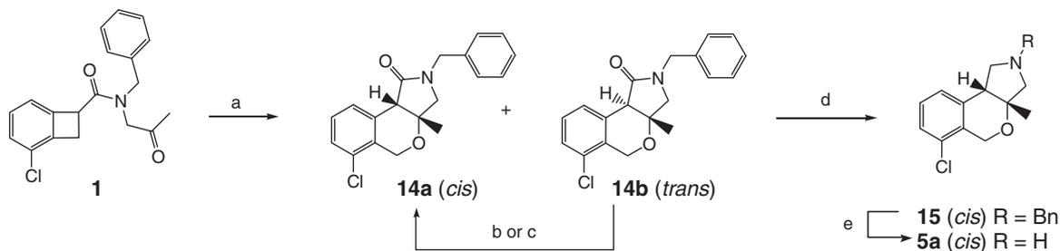
**Scheme 2.** Reagents and conditions: (a) toluene, microwave irradiation, 210 °C, 100%; (b) toluene, microwave irradiation, 220 °C, 100%; (c) DBN, toluene 110 °C, 80%; (d)  $\text{BH}_3$ ·THF, THF, reflux, 4 h, then 2 N HCl, 69%; (e) 1-chloroethyl chloroformate, toluene, reflux, 16 h, then MeOH, 78%.
