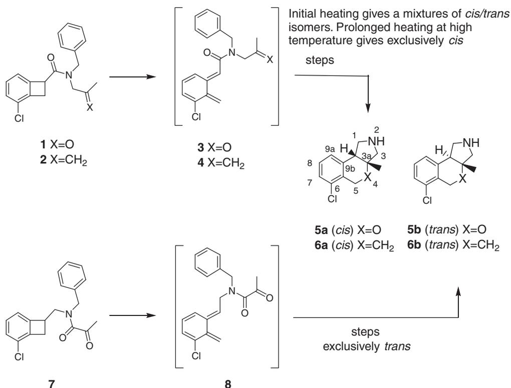
**Figure 1.** Benzocyclobutene intermediates undergo intramolecular (hetero) Diels–Alder reaction proceeding via an *o*-quinodimethane intermediate giving varying ratios of *cis/trans* products depending on the amide position and the tethered dienophile.
