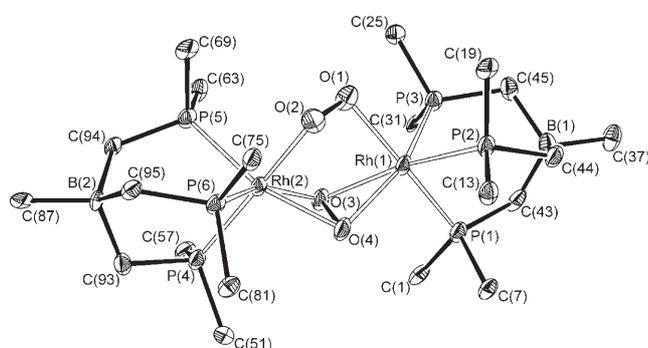
**Figure 2.** ORTEP drawing of **3**. For phenyl substituents, only *ipso* carbon atoms are depicted. Selected bond lengths [Å]: Rh(1)–O(3) 2.125(3), Rh(1)–O(4) 2.144(3), Rh(2)–O(3) 2.151(3), Rh(2)–O(4) 2.132(3).
