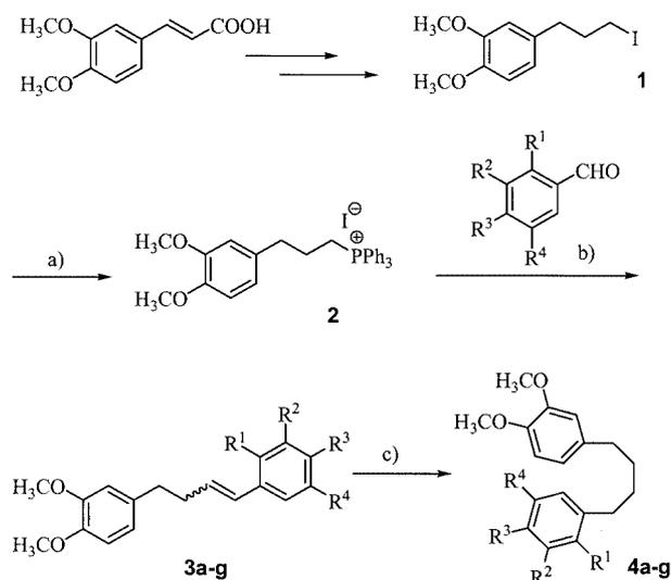
Scheme 1. a)  $\text{PPh}_3$ , DMF, reflux; b) i.  $\text{KO}^t\text{Bu}$ , THF,  $0^\circ\text{C}$ , ii. benzaldehyde derivative; c)  $\text{Pd/C}$ ,  $\text{H}_2$ , THF, room temp.
