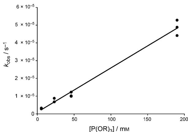
**Figure 2.** Plot of  $k_{\text{obs}}$  ( $\text{s}^{-1}$ ) for approach to equilibrium of *cis/trans*-*P,P*-**5** versus  $[\text{P}(\text{O}-o\text{-tolyl})_3]$  from three separate experiments. For  $[\text{P}(\text{O}-o\text{-tolyl})_3] = 5.6, 23,$  and  $46 \text{ mM}$ , the data points for the separate experiments overlap.
