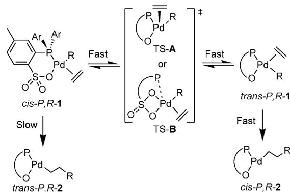
**Scheme 1.** Proposed chain-growth mechanism for  $\{[\text{PO}]\text{PdR}\}$  catalysts.
