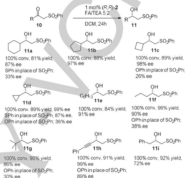
**Figure 4.** ATH of  $\alpha$ -sulfonyl ketones with a tethered ATH catalyst and resulting products **11a-11i**, and comparisons to ees of corresponding ATH products containing sulfides and ethers in place of the sulfone.
