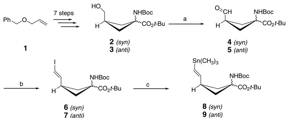
Scheme 1. Syntheses of *syn*- and *anti*-IVACBC stannylated precursors **8** and **9**. Reagents and conditions: (a)  $(\text{COCl})_2$ , DMSO, DCM,  $-50$  °C then  $\text{Et}_3\text{N}$ , 79% (**4**); 64% (**5**); (b)  $\text{CHI}_3$ ,  $\text{CrCl}_2$ , THF,  $0$  °C—rt, 59% (**6**); 60% (**7**); (c)  $(\text{CH}_3)_3\text{Sn-Sn}(\text{CH}_3)_3$ ,  $\text{Pd}^0(\text{PPh}_3)_4$ , THF,  $50$ – $60$  °C, 26% (**8**); 18% (**9**).
