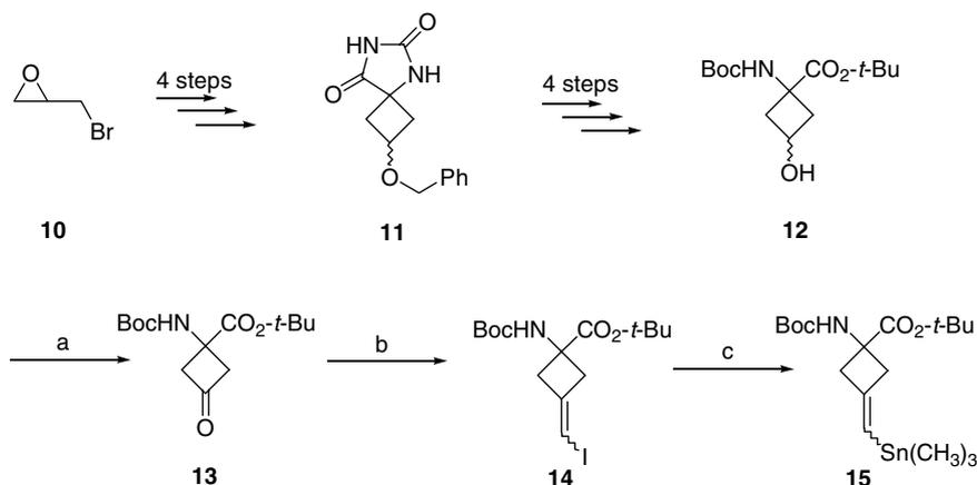
**Scheme 2.** Synthesis of *gem*-IVACBC stannylated precursor **15**. Reagents and conditions: (a)  $(\text{COCl})_2$ , DMSO, DCM,  $-50^\circ\text{C}$  then  $\text{Et}_3\text{N}$ , 92% (**13**); (b)  $\text{CHI}_3$ ,  $\text{CrCl}_2$ , THF,  $0^\circ\text{C}$ —rt, 27% (**14**); (c)  $(\text{CH}_3)_3\text{Sn-Sn}(\text{CH}_3)_3$ ,  $\text{Pd}^0(\text{PPh}_3)_4$ , THF,  $50$ – $60^\circ\text{C}$ , 76% (**15**).
