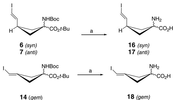
**Scheme 3.** Syntheses of *syn*-, *anti*-, and *gem*-IVACBC **16**, **17**, and **18**. Reagents and conditions: (a) TFA, DCM, rt, 78% (**16**); 71% (**17**); 68% (**18**).
