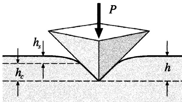
FIG. 1. Total indentation depth  $h$  being the sum of the contact depth  $h_c$  and  $h_s$ .
