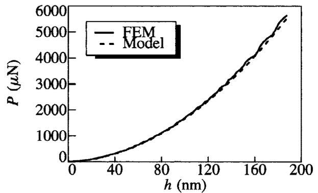
FIG. 4. Indentation load-displacement behavior as computed from FEM and that predicted by the model given by Eq. (12) with the appropriate values substituted for all quantities.
