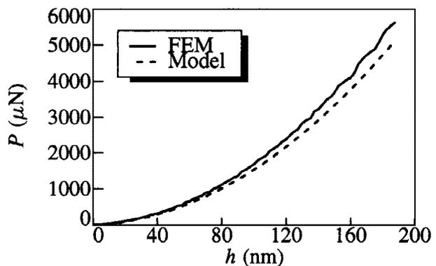
FIG. 5. Indentation load-displacement behavior as computed from FEM and that predicted by the model proposed by Hainsworth *et al.* given by Eq. (2). The appropriate values were substituted for all quantities.
