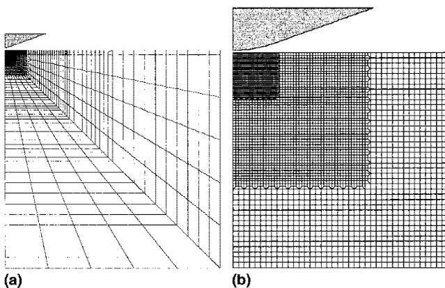
FIG. 3. (a) Full view and (b) detail of the finite element mesh used in the computation. The symmetry axis is on the left side; part of the indenter is visible at the top of the figures.
