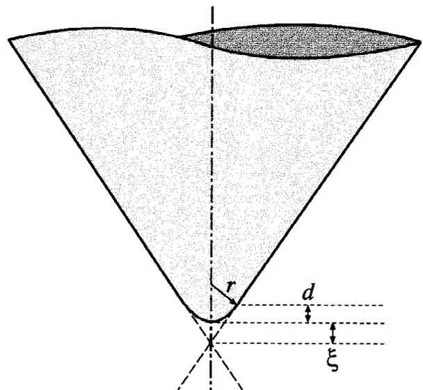
FIG. 2. Schematic diagram showing the geometry of a rounded indenter tip.
