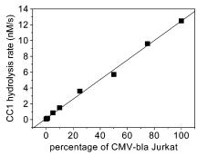
**Figure 2.** Linear dependence of the **CC1** hydrolysis rate on the  $\beta$ -lactamase concentration. Wild-type and CMV-bla Jurkat cells were mixed at different ratios (with the percentage of CMV-bla Jurkat cells from 0, 0.5, 1, 5, 10, 25, 50, and 75 to 100%), lysed, and diluted for CC1 assay with excitation at 365/42 nm and emission at 465/35 nm.
