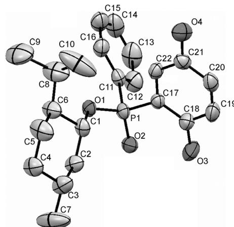
Figure 1. ORTEP drawing of compound (*S*<sub>P</sub>)-**6a**. Hydrogen atoms are omitted for clarity; ellipsoids are drawn at 50% probability. Selected bond lengths [Å] and angles [°]: P1–O1 1.575 (19), P1–O2 1.496 (2), P1–C11 1.790 (3), P1–C17 1.784 (3), C1–O1 1.481 (3), O1–P1–O2 116.11 (11); O2–P1–C17 109.64 (13), O1–P1–C17 109.64 (13), O2–P1–C11 111.70 (13), O1–P1–C11 102.14 (12), C17–P1–C11 109.07 (13), C1–O1–P1 123.87 (17).
