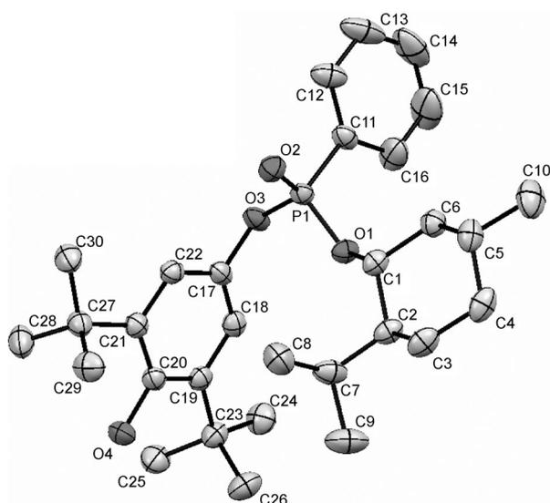
Figure 2. ORTEP drawing of compound ( $S_P$ )-**8b**. Hydrogen atoms are omitted for clarity; ellipsoids are drawn at 50% probability. Selected bond lengths [Å] and angles [°]: P1–O1 1.571 (11), P1–O2 1.470 (12), P1–O3 1.589 (11), P1–C11 1.788 (15), C1–O1 1.473 (18); O1–P1–O2 114.95 (6), O1–P1–O3 102.26 (6), O1–P1–C11 108.86 (7), O2–P1–O3 115.67 (7), O2–P1–C11 112.86 (7), C1–O1–P1 112.36 (9), O3–P1–C11 100.84 (7).
