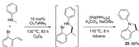
Scheme 1. One-pot synthesis of 3-methyl-*N*-phenylindoline: one-pot TaMe<sub>3</sub>Cl<sub>2</sub>-catalyzed hydroaminoalkylation of *o*-bromostyrene and palladium-catalyzed cyclization.
