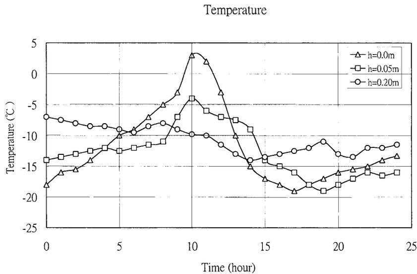
FIG. 3. Calculated Results of Pavement Temperature
