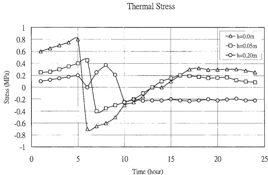
FIG. 4. Calculated Results of Pavement Thermal Stress
