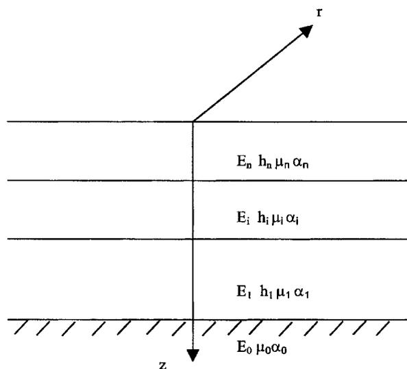
FIG. 1. Calculated Model of Flexible Pavement
