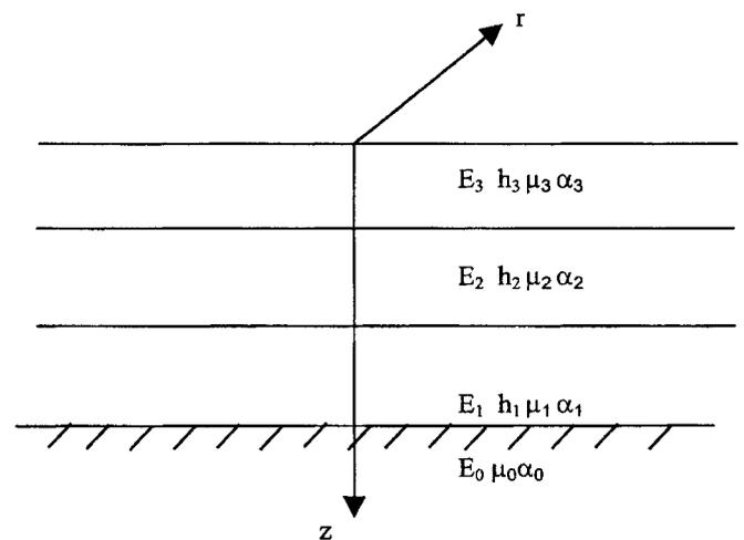
FIG. 2. Computing Model of Practical Pavement
