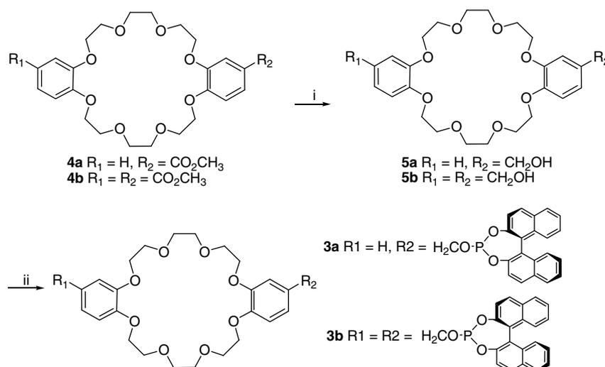
Scheme 1. The synthesis of dibenzo[24]crown-8 host-containing chiral phosphorous ligands **3a** and **3b**. Reagents and conditions: (i)  $H_4AlLi$ , THF, reflux for 2 h; (ii) 2,2'-bisanthol phosphorochloridite,  $Et_3N$ , THF, 16 h, rt.
