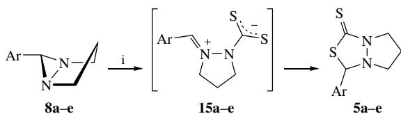
**Scheme 5** Reagents and conditions: i, CS<sub>2</sub> (excess), [bmim][BF<sub>4</sub>] or [bmim][PF<sub>6</sub>], Et<sub>2</sub>O-BF<sub>3</sub>, 20 °C.
