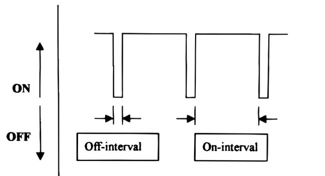
Figure 1. Intermittent electroless nickel deposition process.
