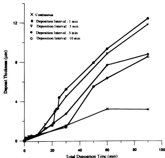
**Figure 4.** Variation of deposition speed with respect to deposition intervals.
