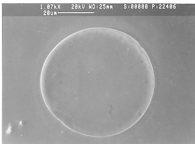
**Figure 3.** Electroless nickel bumps deposited on 60  $\mu\text{m}$  bump pad with on-interval of 5 min.
