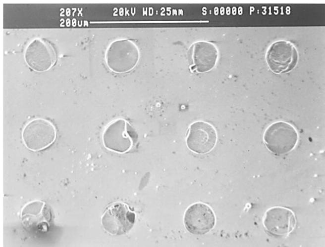
**Figure 2.** Defected appearance of electroless nickel bump deposited on 60  $\mu\text{m}$  bump pad without intermittent.
