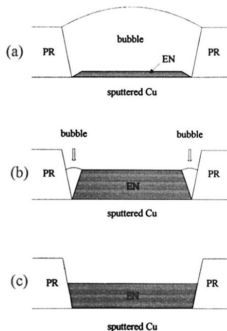
**Figure 5.** The entrapment of hydrogen gas bubble by hydrophobic photoresist opening wall, (a) complete coverage by gas bubble, (b) partial coverage, (c) no entrapment due to intermittent process.
