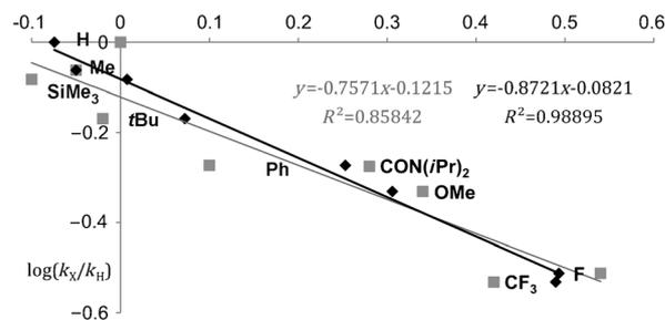
Figure 3. Hammett plot for the arylcyclobutenone rearrangement **1**→**2**+**3** with the  $\sigma_1$  parameter set (■) and with a steric correction ( $\sigma_1-6\% E_s$ , ◆).<sup>[13]</sup>
