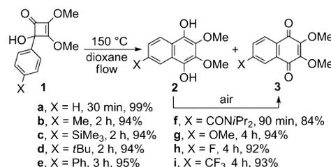
Scheme 1. Arylcyclobutenone rearrangements under continuous flow (with isolated yields quoted for the formation of **3** from **1**).
