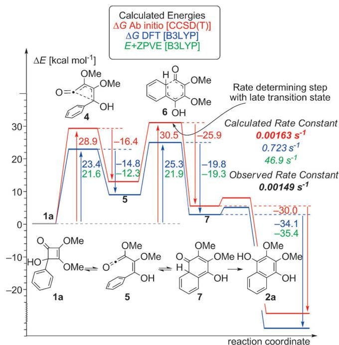
Figure 2. Summary of the energies calculated for the rearrangement **1a**→**2a** in the gas phase at 150 °C computed by  $\Delta(E+ZPE)$  UB3LYP/6-311G(d,p) (in green),  $\Delta G$ (UB3LYP/6-311G(d,p)) (in blue) and  $\Delta G$ (RCCSD(T)/6-31G(d)//UB3LYP/6-311G(d,p)) (in red) as well as associated rate constants.<sup>[15–18]</sup>
