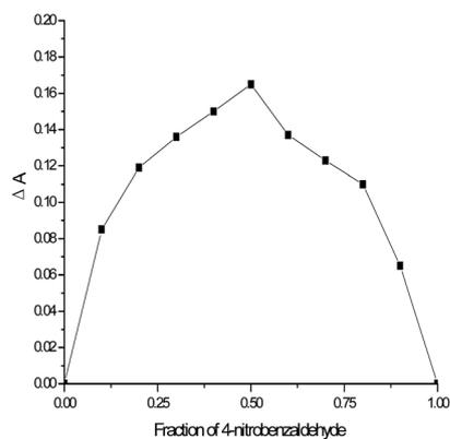
Fig. 4 Job plot for the **a3**/4-nitrobenzaldehyde inclusion system at  $\lambda = 267.5$  nm ( $[\mathbf{a3}] + [4\text{-nitrobenzaldehyde}] = 8.0 \times 10^{-5}$  M) in aqueous  $\text{Na}_2\text{CO}_3\text{-NaHCO}_3$  buffer (pH = 10.5).
