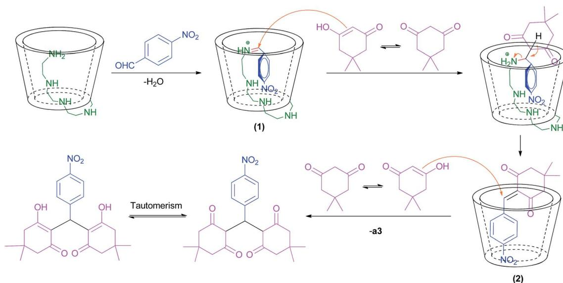
Scheme 3 Possible mechanism for **a3**-catalyzed synthesis of tetraketones.
