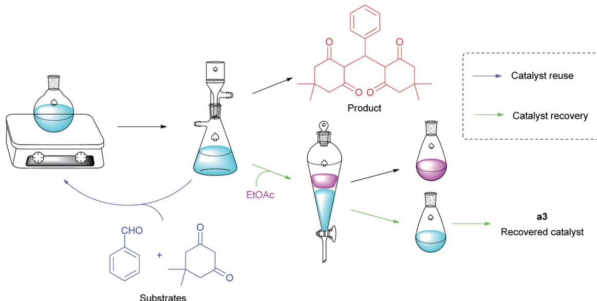
Scheme 4 Process of catalyst (a3) recycling.
