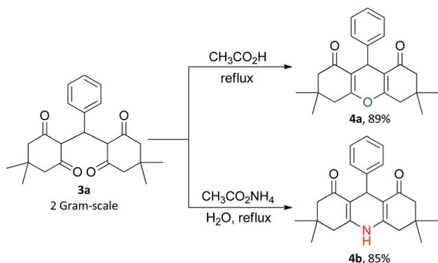
Scheme 5 Gram-scale synthetic applications of tetraketone **3a**.
