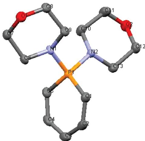
**Figure 4.** The X-ray crystal structure of  $\lambda^5$ -phosphinine **16a**. H atoms were omitted for clarity. Selected bond lengths [Å] and angles [deg]: P(1)–C(1) 1.719, C(1)–C(2) 1.385, C(2)–C(3) 1.390, C(3)–C(4) 1.392, C(4)–C(5) 1.376, C(5)–P(1) 1.718, C(5)–P(1)–C(1) 104.76, N(1)–P(1)–N(2) 99.11.
