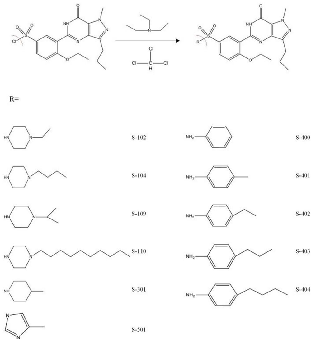
Figure 1. The synthesis pathway of the 11 preferred sildenafil derivatives
