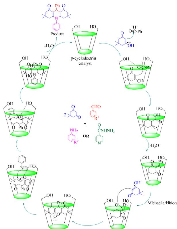
Scheme 3. Plausible mechanism for the synthesis of *N*-substituted 1,8-dioxo-decahydroacridines.
