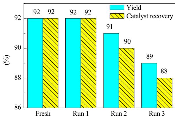
Fig. 2. Reuse and recovery of  $\beta$ -cyclodextrin and its effect on yield.
