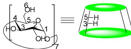
**Fig. 1.** Schematic of the  $\beta$ -CD structure.
