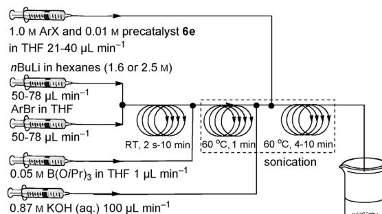
Figure 3. Continuous-flow setup for the lithiation/borylation/Suzuki–Miyaura cross-coupling sequence of two aryl halides.
