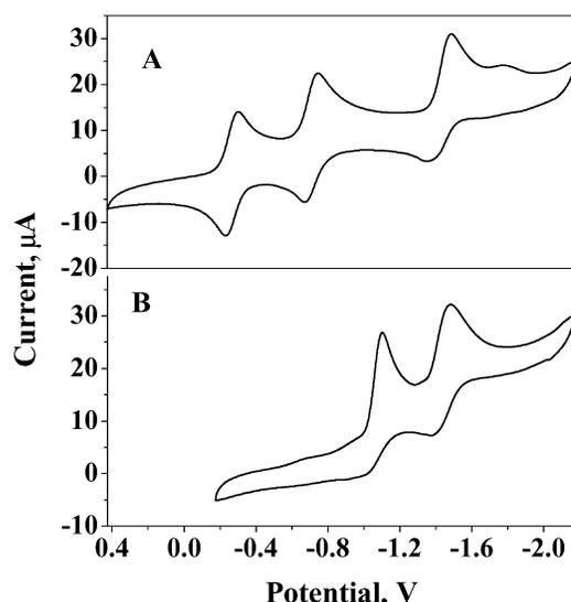
**Figure 4.** Cyclic voltammograms of (A) **1b** and (B) **2b** in acetonitrile showing the reduction peaks.
