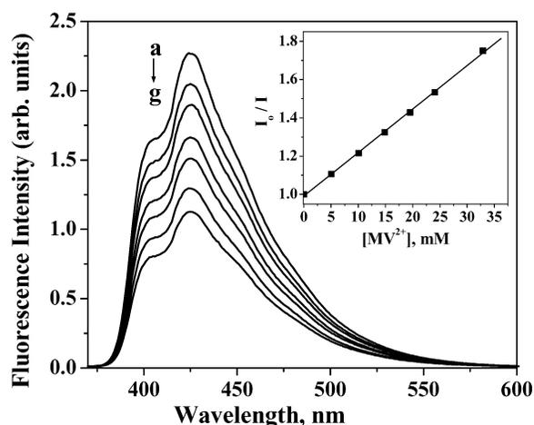
**Figure 5.** Effect of  $MV^{2+}$  concentration on the fluorescence emission spectra of *o*-tolylacridine (**3b**,  $2.9 \times 10^{-5}$  M) in methanol.  $[MV^{2+}]$ : (a) 0; (b) 5.1; (c) 10; (d) 14.8; (e) 24.1; (f) 32.9; (g) 41.3 mM. Inset shows the Stern–Volmer plot for the quenching of **3b** with  $MV^{2+}$ . Excitation wavelength, 355 nm.
