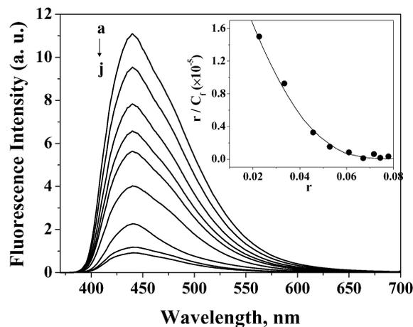
**Figure 9.** Fluorescence emission spectra of **2a** ( $3.7 \times 10^{-5}$  M) in the presence of CT DNA in 10 mM phosphate buffer (pH 8) containing 50 mM NaCl. [DNA]: (a) 0; (b) 0.07; (c) 0.14; (d) 0.20; (e) 0.26; (f) 0.38; (g) 0.5; (h) 0.69; (i) 1.22; (j) 1.5 mM. Inset shows the Scatchard plot for the binding of **2a** to CT DNA. Excitation wavelength, 355 nm.
