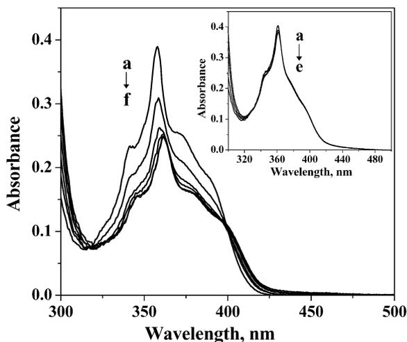
**Figure 7.** Absorption spectra of **1a** ( $3.2 \times 10^{-5}$  M) in the presence of CT DNA in 10 mM phosphate buffer (pH 8) containing 50 mM NaCl. [DNA]: (a) 0; (b) 0.07; (c) 0.14; (d) 0.20; (e) 0.33; (f) 0.44 mM. Inset shows the absorption spectra of **1b** ( $4.4 \times 10^{-5}$  M) in the presence of CT DNA under analogous conditions. [DNA]: (a) 0; (b) 0.14; (c) 0.38; (d) 0.60; (e) 1 mM.
