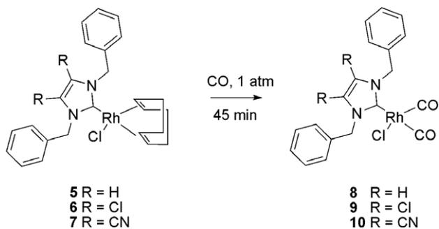
Scheme 7. Synthesis of  $\text{Rh}(\text{CO})_2(\text{NHC})\text{Cl}$  complexes **8–10**.
