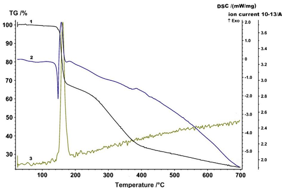
Fig. 2. Thermogravimetric analysis (1), differential scanning calorimetry (2) and mass spectrometric ion current (3, for 167 amu) of compound **4** as a function of the temperature.
