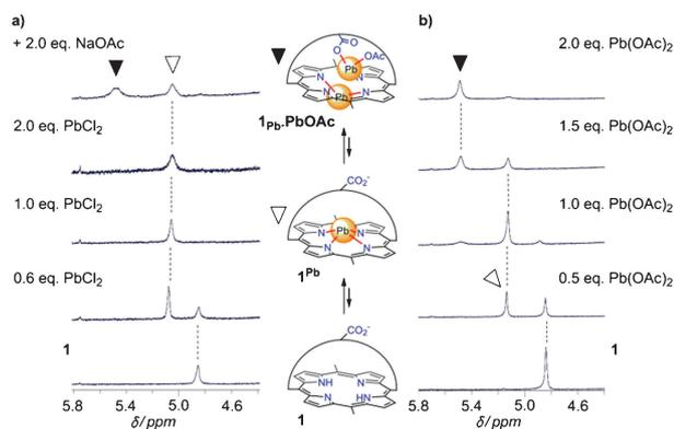
**Fig. 1**  $^1\text{H}$  NMR spectra for the complexation of  $\text{Pb}(\text{II})$  by ligand **1** ( $\text{DMSO}-d_6$ , 500 MHz, 15 equiv. DIPEA, region of the Ha signal). (a) Titration with  $\text{PbCl}_2$ , and subsequent addition of  $\text{NaOAc}$ ; (b) titration with  $\text{Pb}(\text{OAc})_2$ .
