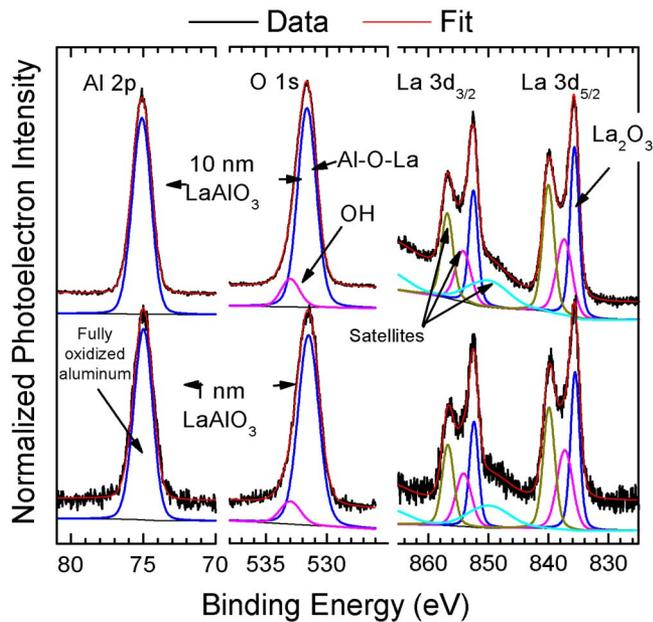
FIG. 3. (Color online) Al 2p, O 1s, and La 3d comparison of 1 vs 10 nm  $\text{LaAlO}_3$  films. There are no detectable differences in the  $\text{LaAlO}_3$  films composition or chemical bonding. The atomic composition calculated from XPS is  $\text{La}_{0.03}\text{Al}_{0.37}\text{O}_{0.60}$ .
