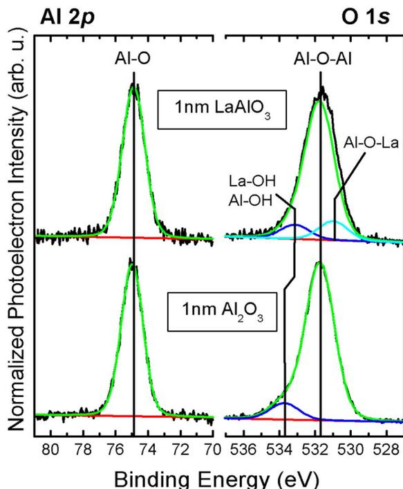
FIG. 1. (Color online) Normalized Al  $2p$  and O  $1s$  XPS peaks for 1 nm of  $\text{LaAlO}_3$  vs 1 nm of  $\text{Al}_2\text{O}_3$ . In both cases Al  $2p$  shows a single chemical component around 74.9 eV corresponding to fully oxidized Al. O  $1s$  shows a main peak around 531.7 eV corresponding to La-O-Al and Al-O-Al bond arrangements for  $\text{LaAlO}_3$  and  $\text{Al}_2\text{O}_3$ , respectively. The small feature at 2 eV above corresponds to hydroxyl groups.
