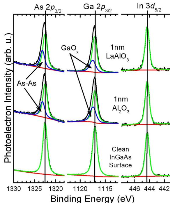
FIG. 2. (Color online) As  $2p_{3/2}$ , Ga  $2p_{3/2}$ , and In  $3d_{5/2}$  showing the surface reaction at the initial growth of  $\text{LaAlO}_3$  vs  $\text{Al}_2\text{O}_3$ . The formation of As-As and Ga-suboxides occurs in a similar manner for the two films. The formation of In oxide is not observed.
