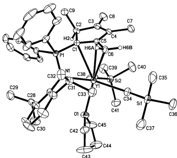
**Figure 4.** X-ray structure of **3a** (40% probability of thermal ellipsoids). Hydrogen atoms are partly omitted for clarity. Selected bond lengths (Å) and angles (deg): C1–C5 1.442(4), C5–C6 1.369(4), C1–C2 1.527(4), C2–C3 1.512(4), C3–C4 1.336(5), C4–C5 1.484(4), P1–C1 1.739(3), P1–N1 1.623(2), Y1–C1 2.749(3), Y1–C5 2.669(3), Y1–C6 2.724(3), Y1–N1 2.383(2), Y1–O1 2.388(2), Y1–C34 2.407(3), Y1–C38 2.408(4); C1–C5–C6 129.9(3), C1–P1–N1 106.2(1), C34–Y1–C38 103.4(2).
