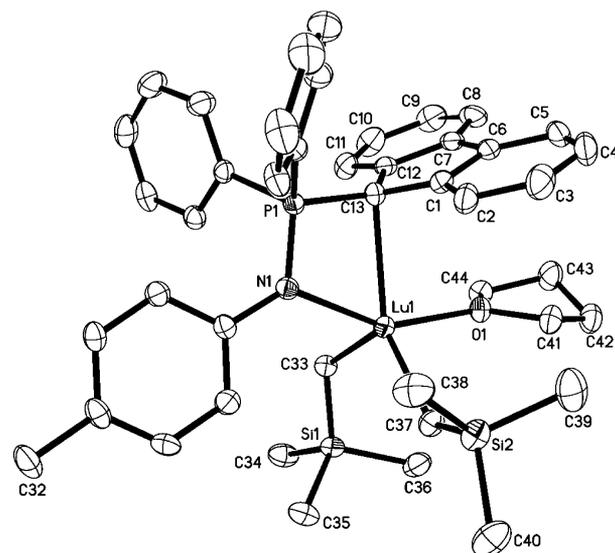
**Figure 10.** X-ray structure of **9b** (40% probability of thermal ellipsoids). Hydrogen atoms are omitted for clarity. Selected bond lengths (Å) and angles (deg): P1–C13 1.752(4), P1–N1 1.612(3), Lu1–C13 2.584(4), Lu1–N1 2.309(3), Lu1–C33 2.320(4), Lu1–C37 2.338(4); C13–P1–N1 104.2(2), C33–Lu1–C37 109.4(1).
