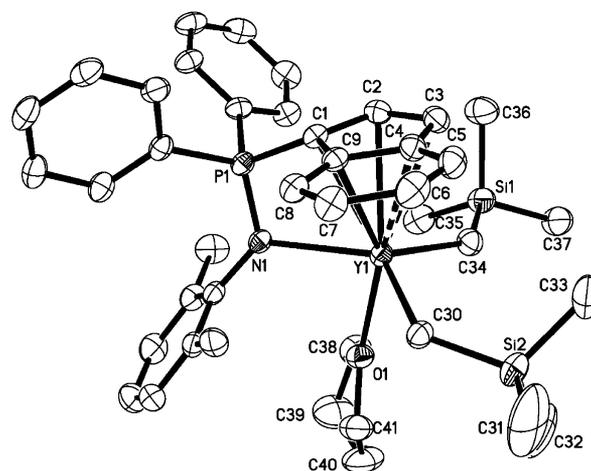
**Figure 7.** X-ray structure of **5b** (40% probability of thermal ellipsoids). Hydrogen atoms are omitted for clarity. Selected bond lengths (Å) and angles (deg): P1–C1 1.755(3), P1–N1 1.603(2), Y1–Cp<sub>cent</sub> 2.538, Y1–C1 2.670(3), Y1–C2 2.759(3), Y1–C9 2.790(3), Y1–C3 2.899(3), Y1–C4 2.935(3), Y1–N1 2.472(2), Y1–O1 2.388(2), Y1–C30 2.404(3), Y1–C34 2.405(3); C1–P1–N1 103.5(1), Cp<sub>cent</sub>–Y1–N1 88.54, C30–Y1–C34 109.8(1).
