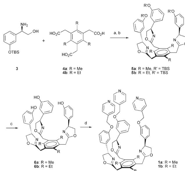
**Scheme 1** Reagents and conditions: (a) (COCl)<sub>2</sub>, Et<sub>3</sub>N, CH<sub>2</sub>Cl<sub>2</sub>; (b) MsCl, Et<sub>3</sub>N, DMAP, CH<sub>2</sub>Cl<sub>2</sub>; (c) 1.0 M aq. NaOH, MeOH, rt, 6 h; (d) NaH, DMF; 4-bromomethylpyridine, CH<sub>2</sub>Cl<sub>2</sub>, rt, 24 h.
